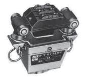
For 30A, 60A ducts 3P 5A trolley. With terminal, Weight 0.7kg.
